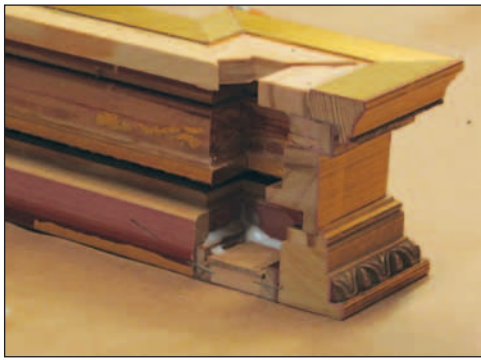
The predella prior to trimming the back edge, showing the filler moulding to set the columns on. (Inset) The back of the predella after all the pieces were cut flush.
