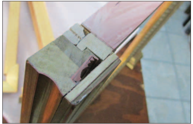
Three individual mouldings make up the entablature or crown of the frame. It is complete at this point, with the exception of filler mouldings on the back
