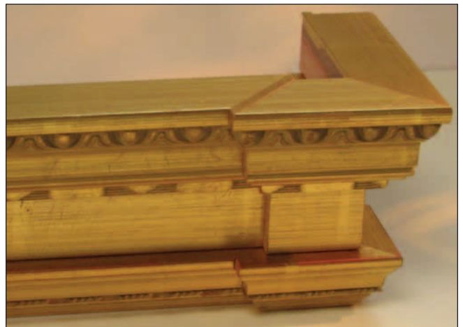
The predella prior to trimming the back edge, showing the filler moulding to set the columns on. (Inset) The back of the predella after all the pieces were cut flush.
