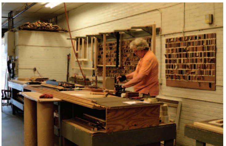
Chip M. Watzulik III joins a frame on the Cassese underpinner in the back-room at the gallery.
