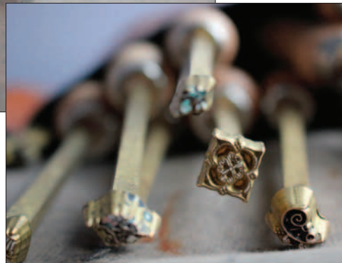
Various metal stamping tools are used to create designs in the surface of the gold leaf, called " granito ." Some tools were adapted for gilding from the leather-working and bookbinding trades.
