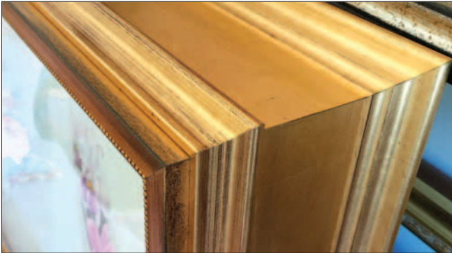
A 5" wide moulding was cut vertically to create the sides of the box frame. The face frame fits neatly inside the gilded rabbet of the box frame.
