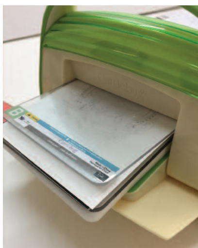
The sandwich was rolled through the Cuttlebug machine twice, once to cut the paper and once to emboss.
