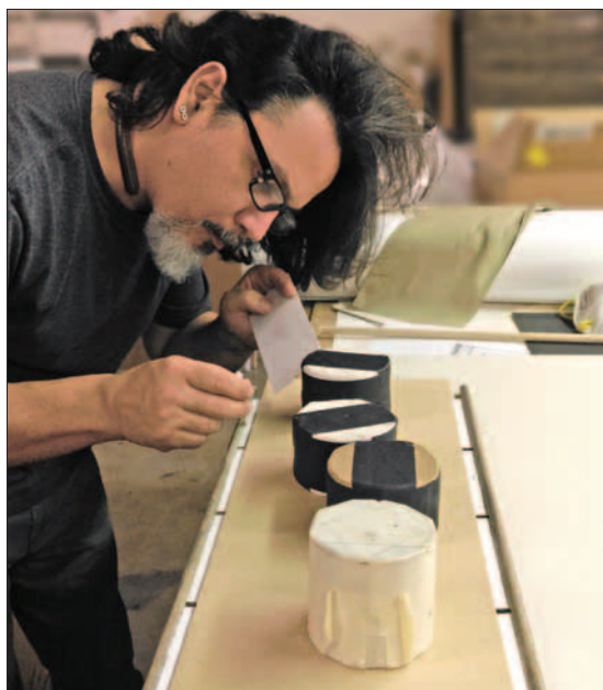
Bonding the scrolls to the fabricated faux bamboo rods.
