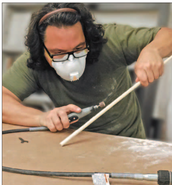
Using a Dremel tool to carve faux bamboo rods from poplar dowels.
