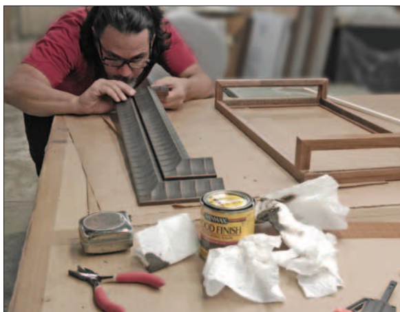
Checking the gap on the double stacked moulding that creates the roof of the tea house.
