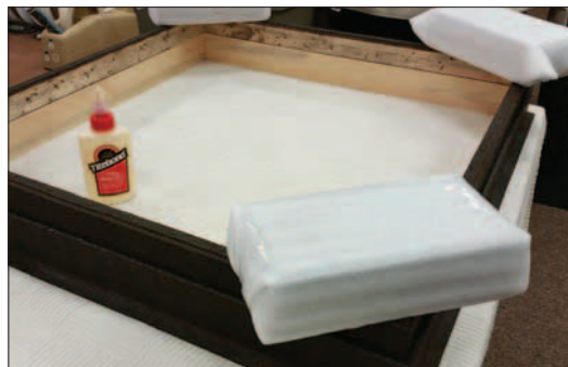
Four padded bricks provided weight to hold the two completed frames in position as they were glued together.
