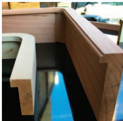
▲ I cut a template to perfect the corners.
