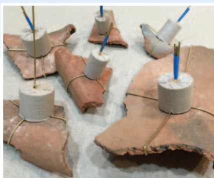
▲ Fabric-covered dowels used for mounting.
