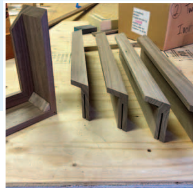
▲ Each section was cut with a table saw.
