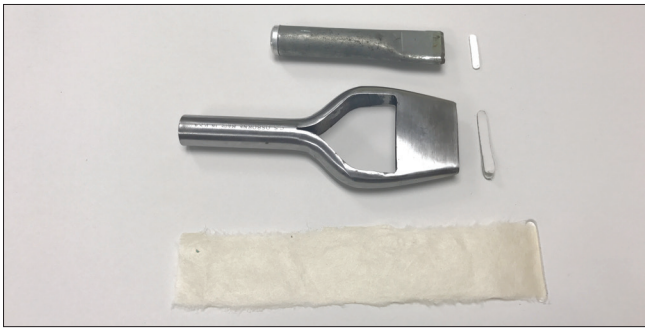
● Cutting the pass-through slot with a leatherworking tool, the slot cutter, which is available in a variety of widths.
