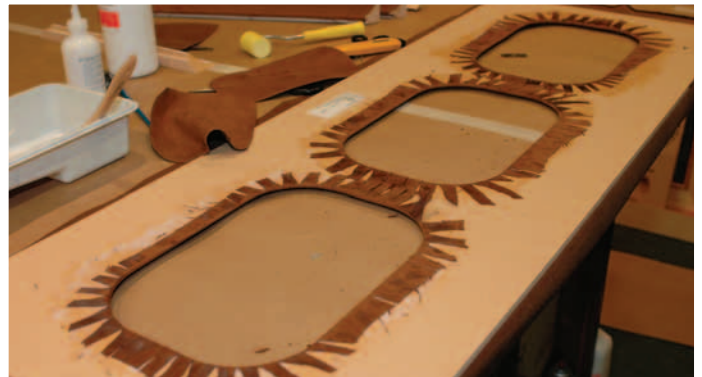
(Bottom right) The back view of the panel liner shows the fabric application process. After fabric has been applied to the front, the center of each window is cut, wrapped around the bevel, and glued to the back.
