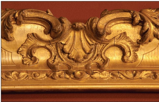
● This frame illustrates the distinctive vertical cracking pattern specific to compo. Courtesy of Suzanne Smeaton
