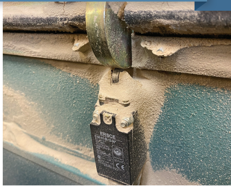
● Sawdust can interfere with the operation of equipment, including this safety cutoff on a double miter saw. Be sure to blow or vacuum off any dust around moving or electrical parts.
