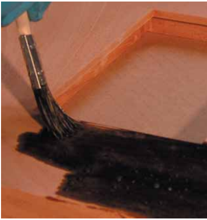
The first coat of stain (natural Watco with a pinch of dark brown pigment added) is applied liberally. Once coated, the frame is left for 15 minutes while the stain is absorbed. Some areas may absorb more than others.
