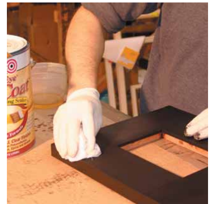
After the ink has dried a thin coat of Zinsser Seal Coat (essentially a clear shellac) is applied with a rag. Depending on the profile used, spraying this coat can yield the best results.
