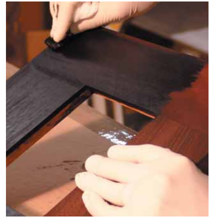
Black Pelikan drawing ink is then applied to the frame with a rag. Be sure to wear gloves for this step as the ink is very hard to wash off.
