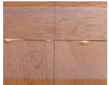
Clear tape is used along the edge of the joint as a mask for the excess glue. This is essential as it prevents the glue from not only getting on the surface (which is easy to remove) but also from the deep pores of the wood. When these are filled with glue it is quite impossible to remove when applying a fine finish.
