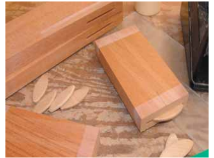
Wood biscuits (compressed beechwood) are inserted into slots with glue for joining. These expand as the joint is left clamped in place.
