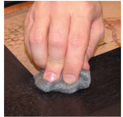
Once the seal coat has dried, typically an hour, it should be buffed with super fine oil-less steel wool to even out any marks from application and to reduce the sheen.
