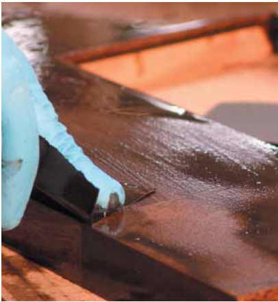
After the first stain has set for 15 minutes a second coat of stain is liberally applied. But this time as soon as the frame is coated it needs to be wet sanded with 400 grit sandpaper, sanding the stain into the finish and creating a slurry of fine dust and stain.
