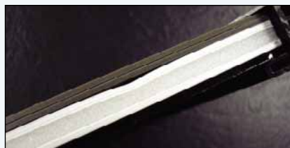
Pressure indentation created by spring clip could be avoided with filler boards.
