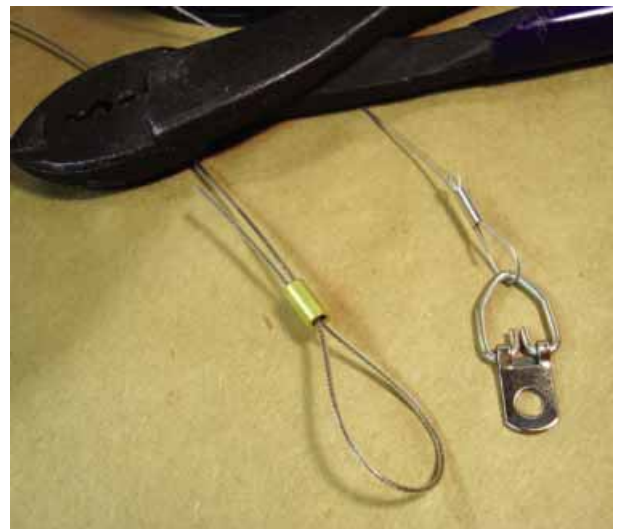
Crimping tool/wire cutter top. Wire is fed through sleeve three times (R) only twice (L).
