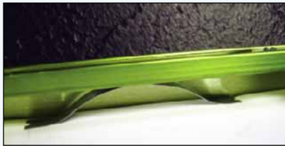
Spring clips are recurve flat metal strips used to press art package to front of frame.
