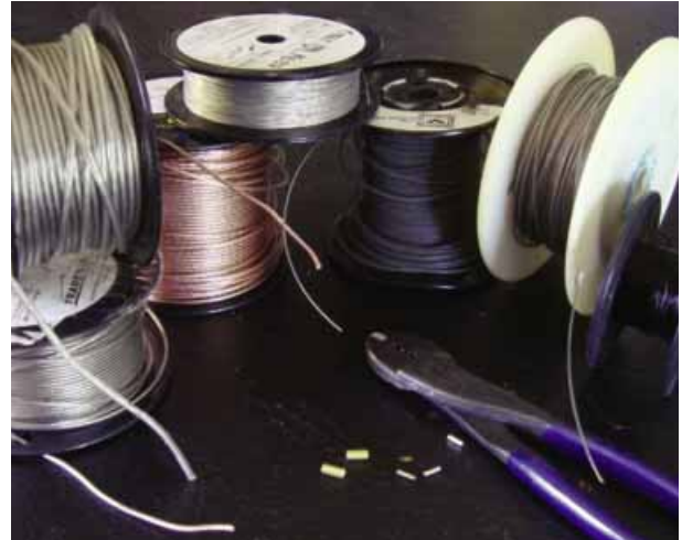
Coated stainless #6 and #8; coated copper #9; stainless #3; braided; and two weights Sevalon sleeve system with crimper tool.
