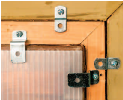
Offset clips come in standard depths and can be easily used to secure canvases in frames without nails.
