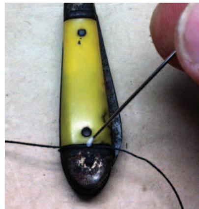
*Pocketknives are double stitched with polyester nylon threads fed through between the body and shell. Getting a tight knot to stay tight when you need to tie the second half of the knot or sew the ends through the backing (as in this case), a very tiny dot of glue on the crossed threads will hold it until you’ve finished whatever else you have to do.*
