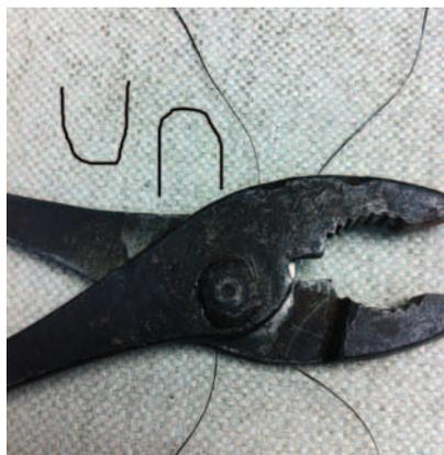
Tools are glued at points, double stitched with polyester nylon threads, as well as bound with Mylar strips. The two U's, when combined between the two halves of the pliers, trap the bolt and then are sewn down in the four reaches, holding the weight and restricting movement. Wrapping Mylar on the handles and passing it through slits to the back keeps the handles from moving.
