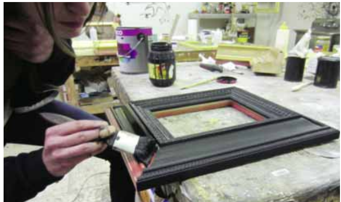
Once the frame is prepared, black supersaturated Rosco paint is brushed on..
