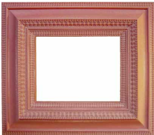
The frame after the red clay undercoat was sprayed on and a thinned shellac sealer was applied.
