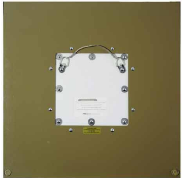
The mounting hardware was attached to the outer frame acrylic backing through a window cut in the floater frame backing.
