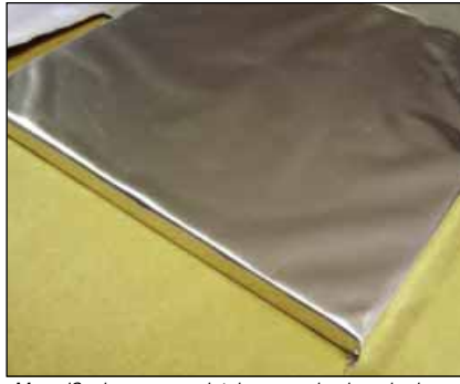
MarvelSeal wrap completely covers back and edges of frame package.
