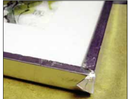
Securely seal corners by ironing in both directions.
