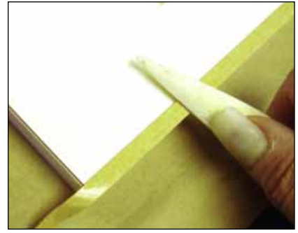
Burnish tape to activate adhesive prior to removing liner.
