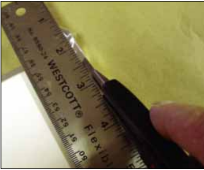
Trim away excess silver film, leaving 1/8" fused film to glass.
