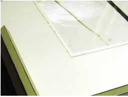
Sealed sandwich includes UV glass, double rag mats with spacer and deckled paper accent and backing glass edge sealed with Marvelseal in an 11x28" Nurre Caxton 3998 Sage moulding.
