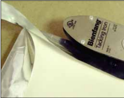
MarvelSeal around edges and stick to tape. Press the flat side of the iron working the full side from corner to corner.
