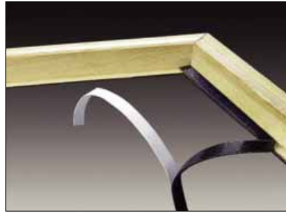
Volara Foam Rabbet Tape is 1/4" wide x 1/32" thick polyethylene closed-cell foam with aggressive acrylic adhesive.
